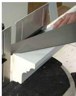
WINDOW SILL PROFILE ANGLED ON BOTH SIDES
